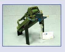
The FROG-4000<sup>™</sup> can be calibrated for a variety of VOCs to include benzene, toluene, TCE, PCE, and many other VOCS. The instrument display will inform the user which VOCs are detected and their concentration. An on-board SD card stores all of the data the FROG-4000<sup>™</sup> has acquired and that data can be downloaded to a computer later.
