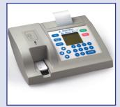
Defender TSR (Test Strip Reader) a hand-held optical reader. A protein detection test is also part of the system.
