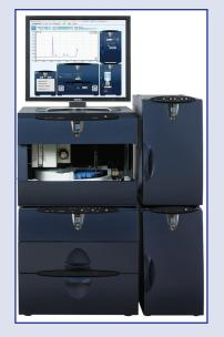
Free IC systems with Eluent Regeneration (RFIC-ER systems) are designed to use carbonate, carbonate/bicarbonate, or MSA eluents for isocratic separations. Eluent Regeneration is available as an optional configuration or upgrade for ICS-1100, -1600, -2100, and -5000 systems.
