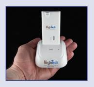
pathogen targets, subtypes, antibiotic resistance from sample-to-answer in <45 minutes. The readout module can either be simple colorimetric Yes or No answers, or digital quantitative readout via the use of a cell phone-sized reader. The data collected from the diagnostic device has the option to be submitted to the remote data processing center via wireless or secure data transferring methods. The device has the option to be run on batteries or regular AC electricity outlets.
