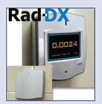
they are in range of a single Rad-DX system (up to 1000 meters)! The Rad-DX units will automatically form an intelligent, self-healing mesh network, allowing them to be constantly connected to each other as well as to the user network.
