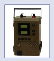
equipped with an automatic overload protection system. The radiation sensor is calibrated once before delivery to the customer. After this initial calibration, no further calibration is required.
