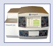
buccal swab samples and sample processing is initiated with no further user interaction. The system extracts DNA from the samples and performs STR amplification, electrophoretic separation and software analysis to generate full DNA profiles in about 90 minutes. For the U.S. market, the results data are saved in CODIS-compatible format within the embedded GeneMarker HID® software (SoftGenetics®, LLC). Other data formats will be available as needed.
