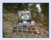
The Ship Ballast CBRN Solar Powered Water Monitor – Portable, MiniTect, contains 20 sensors detecting radiation, microorganisms, and chemicals.
