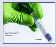
sample tip on the suspect material; analyze the sample by cracking the builtin ampoules and watching for the specified color change.
