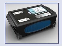
the user introduces a swab of unknown material into the system, the unit will automatically perform the steps of sample recovery, lysing, purification, real-time PCR amplification, and fluorescence detection in order to determine if the material contains genetic material with a sequence matching an on-board library of known threats.
