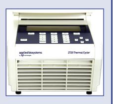
( $\pm 0.25^{\circ}$ C from 35°C to 100°C) and long term stability and high reliability. The sample block accommodates several different types of MicroAmp® disposable tubes and plates, which must be used in order to create a sealed chamber.
