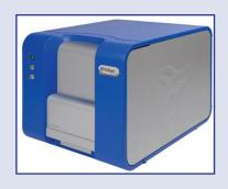
microfluidics technology the LabChip GXII eliminates the need to handle time consuming SDS page gels, and provides superior results for less time and money.
