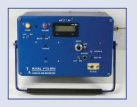
programmable digital readout; sensitive for occupational exposure dynamic background compensation; battery operation or ac operation; built-in high level alarm; built-in low flow alarm; built-in RS-232 computer interface. End Users: nuclear power plants, coal fired power plants, pharmaceutical labs, universities.
