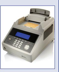
range (4°C to 99.9°C), accurate measurements ( $\pm 0.25$ °C from 35°C to 100°C) and long term stability and high reliability.
