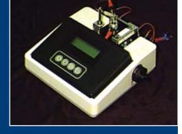
transfer (FRET) reader, capable of rapid one-step immunoassays (without wash steps). Immuno FRET assays were developed for Bacillus cereus spores and E. coli bacteria (see Bruno et al., Biochem. Biophys. Res. Comm. Vol. 287:875-880, 2001). Assays are currently performed in 50 uL plastic or silicon cartridges, OmniSite is developing microfluidic cartridges that will contain freeze-dried immuno-FRET reagents that can be rehydrated by the sample and assayed within minutes.
