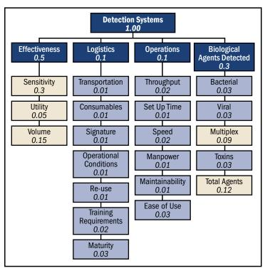
Figure 5. Hierarchical representation of criteria for Evaluation of Detection Products for Analytical Laboratories
