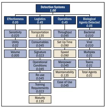
Figure 2. Hierarchical representation of criteria for Evaluation of Detection Products for Field Use
