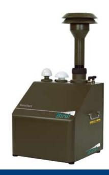
measuring the size and shape of individual particles and measuring the fluorescence response of an aerosol sample. This information is combined using powerful analytical tools to interpret with a high degree of confidence whether an aerosol is biological or non biological. Its response is real time providing field commanders and first responders with an early warning capability to enable evasive action or appropriate protection measures to be undertaken.
