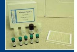
the quantification of Aflatoxin residues in grains and grain-based products. The limit of detection is two parts per billion. A ground sample is extracted by shaking with a 70% methanol solution. This extract is filtered and then analyzed in the immunoassay along with calibrator solutions of known Aflatoxin concentration and the Aflatoxin content of the sample is derived. The total assay time is less than 20 minutes.
