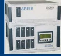
detection. The newly developed APSIS is an identifier for harmful pathogens, like bacteria, spores and viruses, based on their genomic fingerprint stored in their DNA or RNA. The system is intended for the on site analysis of microorganisms (bacteria, spores and viruses) in mobile labs and onboard vehicles. The performance is not limited to harmful pathogens used as BWA but also covers pathogens for clinical diagnostic purposes.
