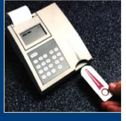
fluorometer to read the ticket. Triage measures multiple analytes simultaneously in any biological fluid using a single ticket, which makes it possible to simultaneously identifying all BW threat agents on one ticket. Biosite has also developed a highly specific (low false alarm rate) and sensitive immunoassay on Triage for the detection of Bacillus anthracis.
