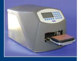
DNA, DNA sequencing, and other applications requiring rapid changes in temperature. The system is based on a new patented technology that allows for both high speed thermal cycling and high density work. The system is the only thermal cycler currently available that will work with both 384 well plates and 1536 well plates with sample volumes as low as one microliter.
