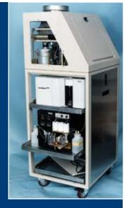
profile targets in which the public is at high risk to bioterrorist attacks. The APDS is completely automated, offering aerosol sampling, in-line sample preparation fluidics, and orthogonal immunoassay and nucleic acid detection device. This system has flexibility, cost, and system performance and should be compared to competing technologies.
