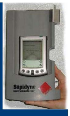
the Handheld are investigating its application for the detection of heavy metals in solution utilizing antibodies developed by Dr. Blake. The beta unit of the handheld is controlled by a hand held computer for ease of transport, field operation, and data transfer.
