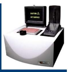
Palm-Cycler is used to facilitate the enzymatic reactions necessary for many detection methods. It does not directly detect anything itself. There are a wide array of sequencing, DNA amplification, Real-Time and isothermal reaction assays that can be used on the Palm-Cycler.
